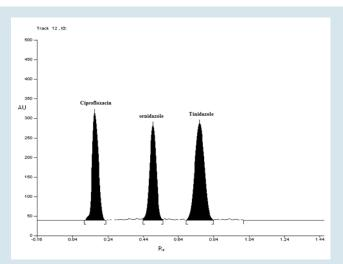
**Figure 3:** Densitogram of ciprofloxacin 100 ng/spot (Retention factor =  $0.18 \pm 0.0057$ ), ornidazole 100 ng/spot (Retention factor = $0.49 \pm 0.0057$ ), tinidazole (IS) 100 ng/spot (Retention factor  $0.75 \pm 0.0054$ ).
