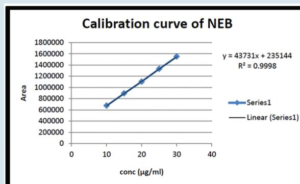
Figure 6b: Calibration curve for NEB in HPLC method.
