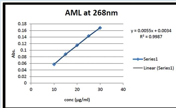
Figure 4b: Calibration curve of AML at 268 nm.
