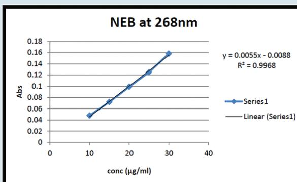
Figure 4d: Calibration curve for NEB at 268 nm.
