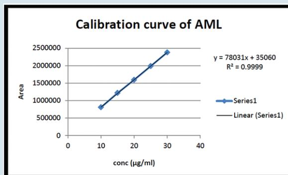
Figure 6a: Calibration curve for AML in HPLC method.
