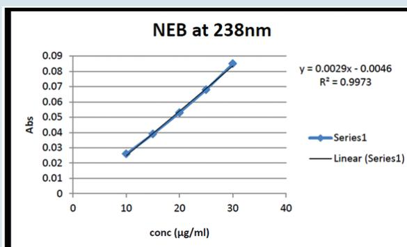
Figure 4c: Calibration curve for NEB at 238 nm.
