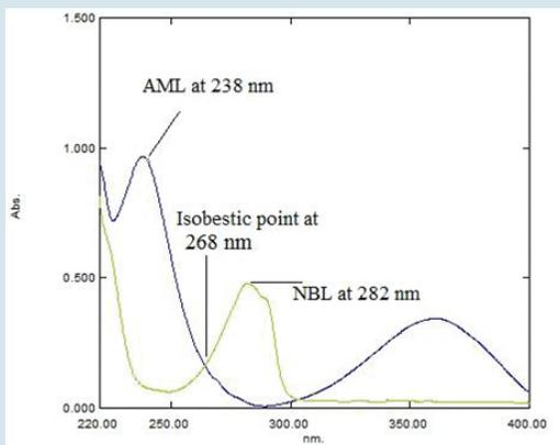
Figure 3: Overlay UV-spectra of AML and NEB.
